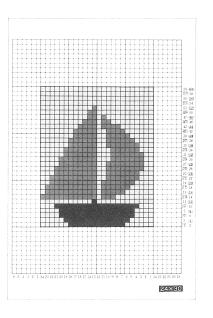
To punch a card for Double Jacquard using a blank card it is important to realise that each row of Double Jacquard pattern consists of two rows of slip stitch knitting. One is with background yarn and the other is with contrast yarn.
