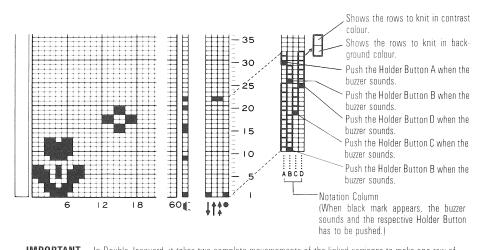
**IMPORTANT** In Double Jacquard, it takes two complete movements of the linked carriages to make one row of finished knitting on the main bed. The light by Pattern Switch 1 shows whether you are knitting background (right) or contrast (left).
