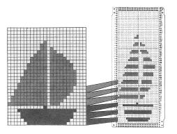
(2) Mark the parts of contrast yarn on the first and second rows of the pattern onto the second and third rows of the Card (non-coloured rows) respectively.
